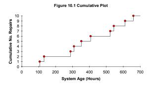
Under a renewal process, the times between failures are i.i.d., that is, from a single population having a fixed mean (average) repair time. Consequently, the cumulative plot should appear to follow a straight line.
