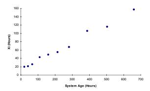
Now the order in which the interarrival times appear is important. Again we confirm an improving trend. We cannot use standard non-repairable methods, such a probability plotting, to analyze such data by assuming the time between repairs are independent observations from a single population.
