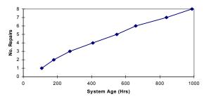
The engineers analyzed the repairable system data in a traditional manner (See Tobias and Trindade.) by taking times-between-repairs and treating them as a group of independent and identically distributed observations arising from a single population of failure times. Methods for the analysis of nonrepairable components were used including Weibull probability plotting of data, parameter estimation, and model fitting. Thus, the times between repairs (called the
